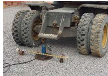
7. Load plate test(φ450mm)
